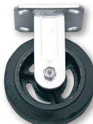
WH 53 6" X 2" Mold-On Rubber Rigid Plate 4" X 4 1/2" 410 lbs. Cap. Wt. 6 1/4 lbs.
