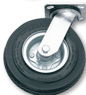
WH 96 8" X 2 1/2" Pneumatic Swivel Plate 4" X 4 5/8" 250 lbs. Cap. Wt. 6 1/2 lbs.
