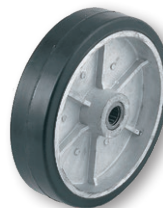
WH 73 8" X 2" Mold-On Rubber 3/4" Roller Bearing 2 1/4" Hub Width 450 lbs. Cap. Wt. 3 1/2 lbs.
