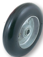
WH 55 8" X 2 1/4" Balloon Cushion 5/8" B.B. 2" Hub Width 350 lbs. Cap. Wt 4 lbs.
