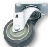
WH 46 3 1/2" X 1 1/4" Mold-On Polyurethane Swivel Plate 2 3/8" X 3 5/8" 200 lbs. Cap. Wt. 1 3/4 lbs.
