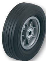
WH KB01 10" X 3 1/2" Micro Cellular Foam Polyurethane 5/8" B.B. 2 1/4" Hub Width 300 lbs. Cap. Wt. 3 1/2 lbs.
