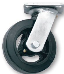
WH 51S 6" X 2" Mold-On Rubber Swivel Plate 4" X 4 1/2" 410 lbs. Cap. Wt. 7 1/4 lbs.
