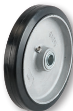
WH 61 8" X 1 5/8" Mold-On Rubber 3/4" B.B. 2" Hub Width 450 lbs. Cap. Wt. 2 1/4 lbs.
