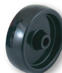
WH 63P 6" X 2" Polyolefin 5/8" Plain 2 1/4" Hub Width 750 lbs. Cap. Wt. 1 lb.
