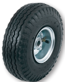
WH 19 10" X 3 1/2" Pneumatic 3/4" B.B. 3 1/4" Hub Width 350 lbs. Cap. Wt. 4 lbs.
