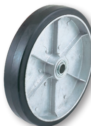
WH 62 10" X 2" Mold-On Rubber 5/8" B.B. 2 1/4" Hub Width 600 lbs. Cap. Wt. 5 1/2 lbs.
