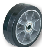
WH 63 6" X 2" Mold-On Rubber 5/8" B.B. 2 1/4" Hub Width 460 lbs. Cap. Wt. 2 1/4 lbs.
