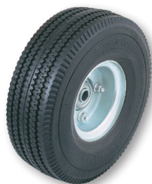
WH KB01 10" X 3 1/2" Micro Cellular Foam Polyurethane 5/8" B.B. 2 1/4" Hub Width 300 lbs. Cap. Wt. 3 1/2 lbs.
