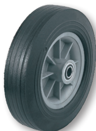
WH 83 10" X 2 1/2" Solid Crumb Rubber 3/4" B.B. 3 1/4" Hub Width 400 lbs. Cap. Wt. 6 lbs.
