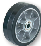
WH 67 6" X 2" Mold-On Rubber 3/4" B.B. 2 1/4" Hub Width 460 lbs. Cap. Wt. 2 1/4 lbs.
