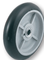
WH 56P 8" X 2 1/4" Balloon Cushion 3/4" B.B. 2 1/4" Hub Width 400 lbs. Cap. Wt. 2 3/4 lbs.
