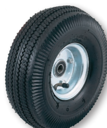
WH 16 10" X 3 1/2" Pneumatic 5/8" B.B. 2 1/4" Hub Width 350 lbs. Cap. Wt. 4 lbs.
