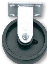
WH 54 6" X 2" Polyolefin Rigid Plate 4" X 4 5/8" 820 lbs. Cap. Wt. 4 lbs.
