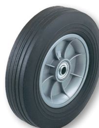
WH 60 10" X 2 1/2" Solid Crumb Rubber 5/8" B.B. 2 1/4" Hub Width 400 lbs. Cap. Wt. 5 1/2 lbs.
