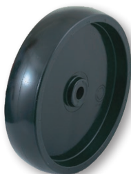
WH 68P 10" X 2 1/4" Polyolefin 3/4" Plain 2 1/4" Hub Width 1000 lbs. Cap. Wt. 2 1/2 lbs.
